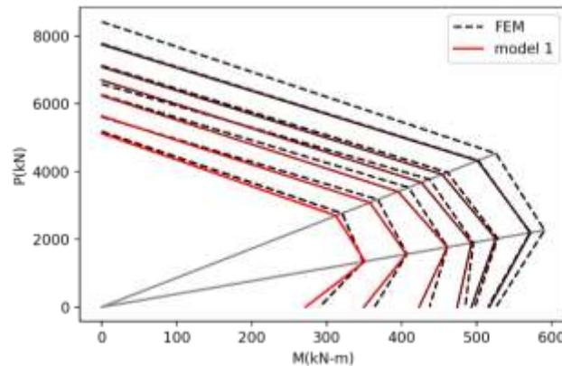
Fig. 3 example of LGBM reconstructed P-M interaction diagram (B=36, H=54, BN=2, HN=10)
