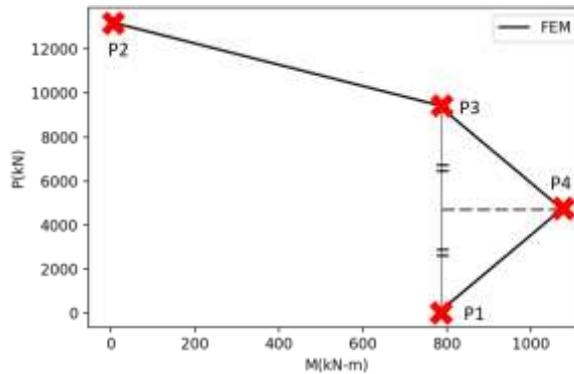
Fig. 2 P-M interaction reduction to 4 core points
